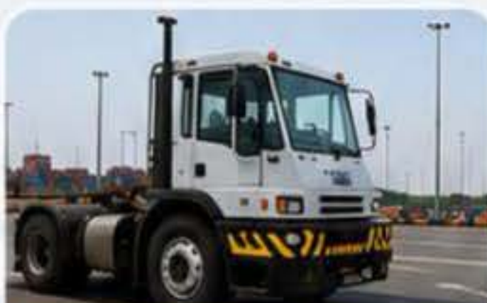
TRUCK BOT (TERMINAL TRACTOR)
